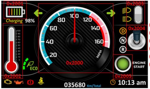
0x2000 Gauge 0x2001 Battery 0x2002 Temperature 0x2003 Toggle Button 0x2004 Toggle Button 0x2005 Indicator
